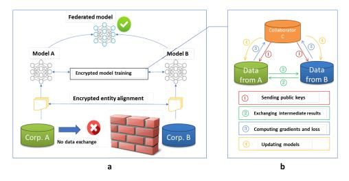
Fig. 4. Architecture for a vertical federated learning system
